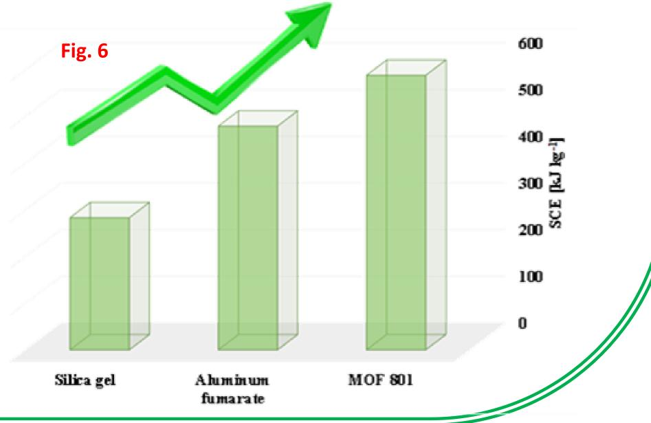
N.B. For Fig. 5 and 6, Cooling temperature was considered as 283K while having 343K as
