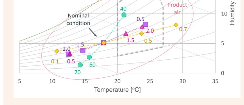
*Effect of varying regeneration temperature, channel length, air velocity, and product air extraction ratio to product air minimum temperature & humidity in CoDECS.*
