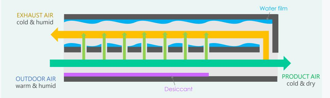
Combined desiccant dehumidification and dew point evaporative cooling system (CoDECS).
