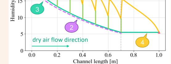
Temperature and humidity distribution along the dry and wet channels of CoDECS at nominal operating condition and t = 500s.
