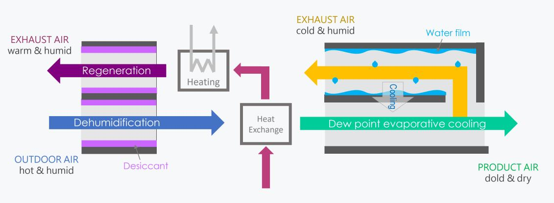
Independent desiccant dehumidification and dew point evaporative cooling.
