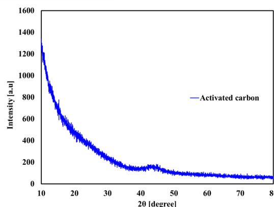
Fig 4: XRD pattern of activated carbon
