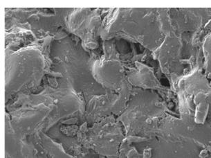
Fig 3: SEM image of activated carbon
