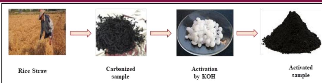
Fig 2: Synthesis steps of activated carbon
